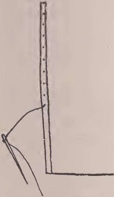
Fig. (71) Roll the joining of the seam onto the wrong side of the coat
